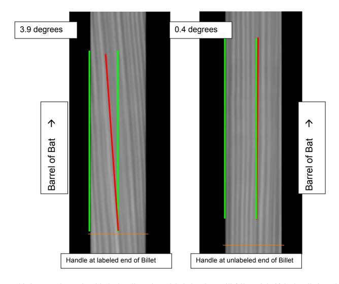
This bat <u>must</u> be made with the handle at the unlabeled end. It will fail outright if the handle is at the unlabeled end.
