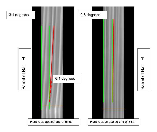
This bat <u>must</u> be made with the handle at the unlabeled end. It will fail the ink spot test if made with the handle at the labeled end. Further, a sharp bend in the grain at that end may act as a stress concentrator, making the bat more likely to fracture.
